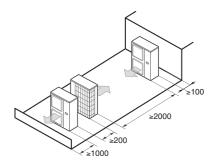
In case of installing multiple units (2 units or more) in lateral connection per row.
