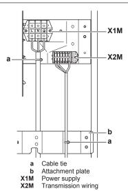
5 Route the wiring through the frame and connect it to it.
