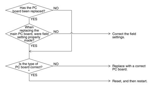
\*Note) Type of PC board mismatching includes; Main PC board Inverter PC board (for compressor) Fan driver PC board
