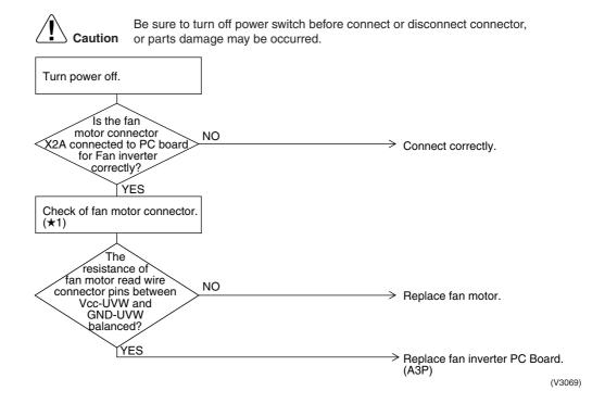
★1: Disconnect connector (X2A) and measure the following resistance.
