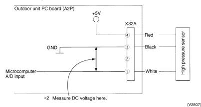
\*2: Refer to "Pressure Sensor, Pressure / Voltage Characteristics" table on P367.
