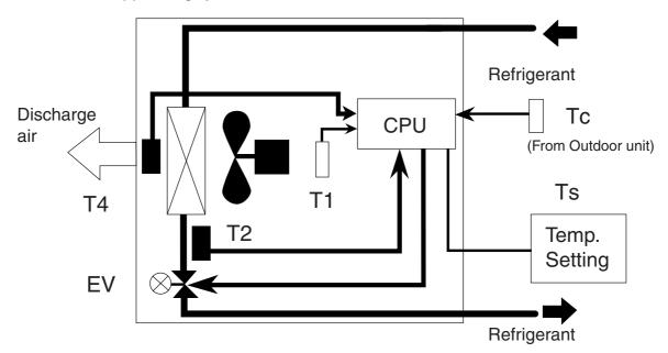
T1: Temperature detected by suction air thermistor Th1
