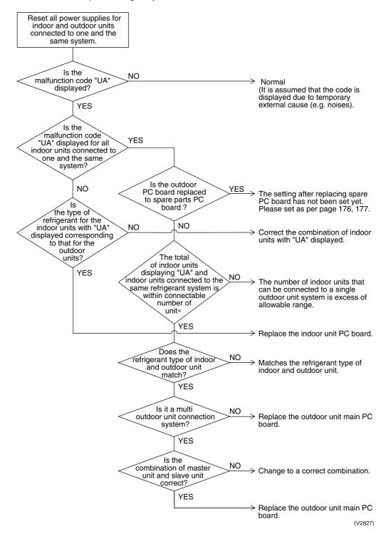
\* The number of indoor units that can be connected to a single outdoor unit system depends on the model of outdoor unit.
