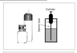
Refrigerant can be charged in liquid state with cylinder in upright position.
