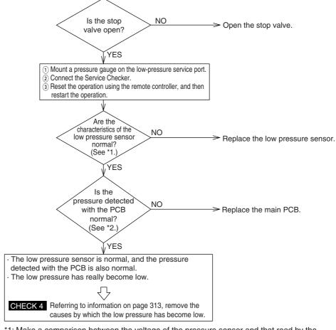
\*1: Make a comparison between the voltage of the pressure sensor and that read by the pressure gauge.
