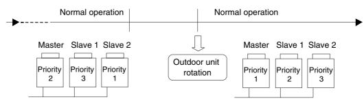
\* "Master unit", "slave unit 1" and "slave unit 2" in this section are the names for installation. They are determined in installation work, and not changed thereafter. (These names are different from "master unit" and "slave unit" for control.)
