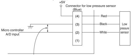
Make measurement of DC voltage between these wires.
