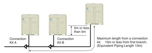
Since there is a possibility that oil may be collected on a stop machine side, install piping between outdoor units to go to level or go up to an outdoor unit, and to make a slope.
