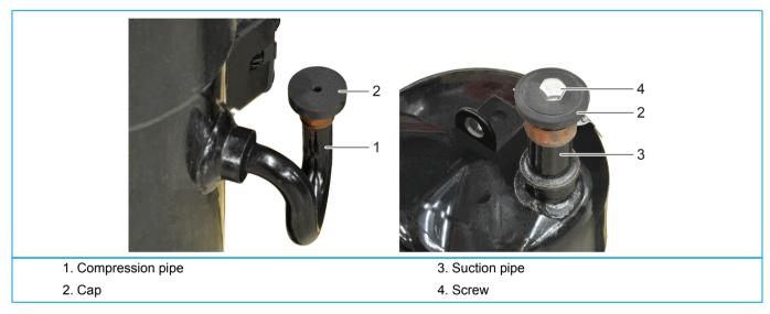
5. Insert a lint-free cloth (3) into the compression pipe (2) to lower the oil in the compression pipe to the indicated oil level (4).
