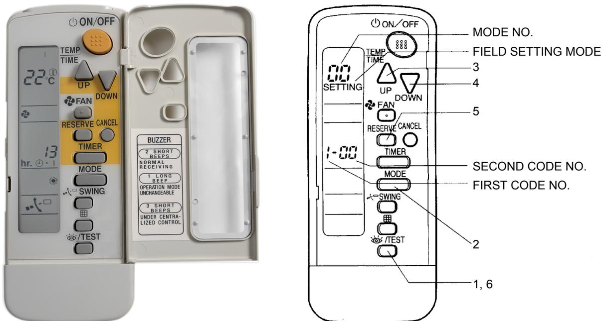
1. When in the normal mode, press the “
