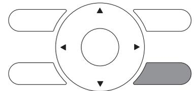
Press and hold the Cancel button for 4 seconds or longer while the backlight is lit.
