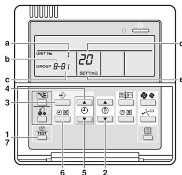
1. When in the normal mode, press the “
