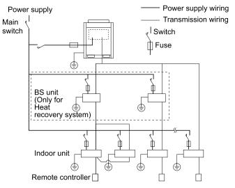
1. When using 1 remote controller for 1 indoor unit. (Normal operation)
