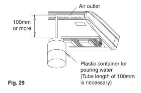
After the drain piping work, install the stay for packing and delivering (reinforcing plate), which was removed in the section of "6. REFRIGERANT PIPING WORK".
