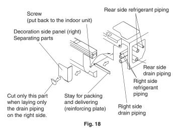
• After piping is finished, cut the removed penetration cover along the shape of piping, and install.
