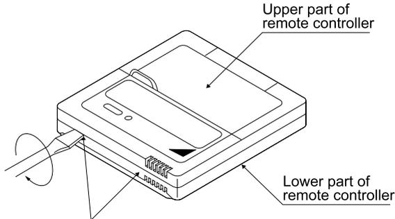
Insert the screwdriver here and gently work off the upper part of remote controller.
