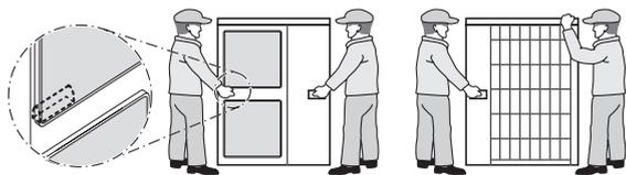
Place your hands on the corner instead of holding the suction inlet in the side of the casing, otherwise the casing could be deformed.
