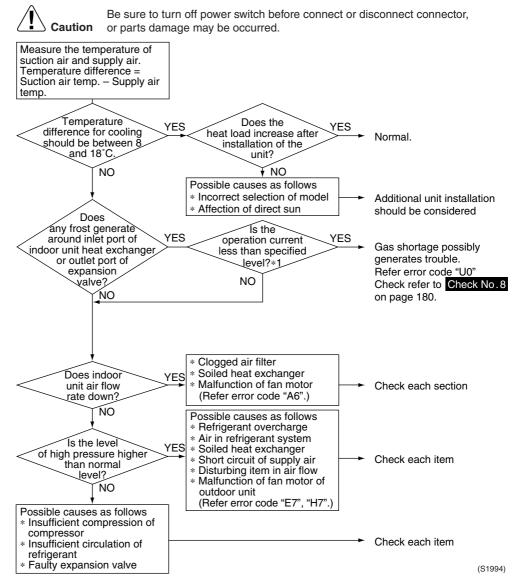
\*1: For operating current, refer to "Electric characteristics" (on page 9) after checking the field system combination (indoor + outdoor).
