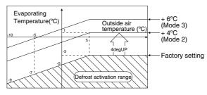
When defrosting conditions are met during heating operation, the indoor unit is demanded defrosting and the following control is performed:
