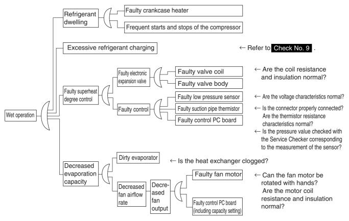
Referring to the Fault Tree Analysis (FTA) shown below, identify the faulty points.
