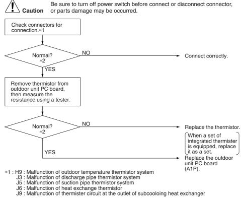
★See Check No. 6 for "Thermistor temperature/Resistance characteristics".
