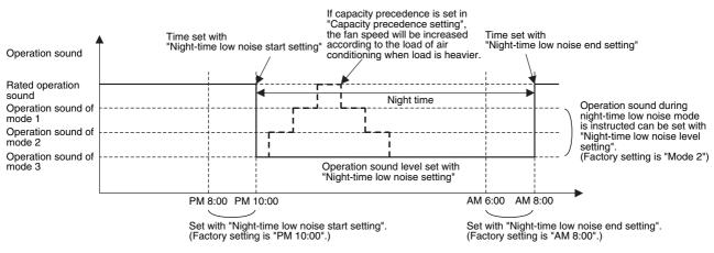
\* "Start time" and "End time" must be regarded as a guide because they are estimated based on the outside air temperature.
