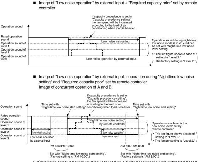
\* "Start time" and "End time" must be regarded as a guide because they are estimated based on the outside air temperature.
