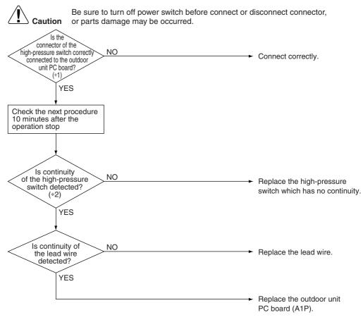
\*1. The connector No. of the high-pressure switch (protection from high-pressure) is shown in the following table.
