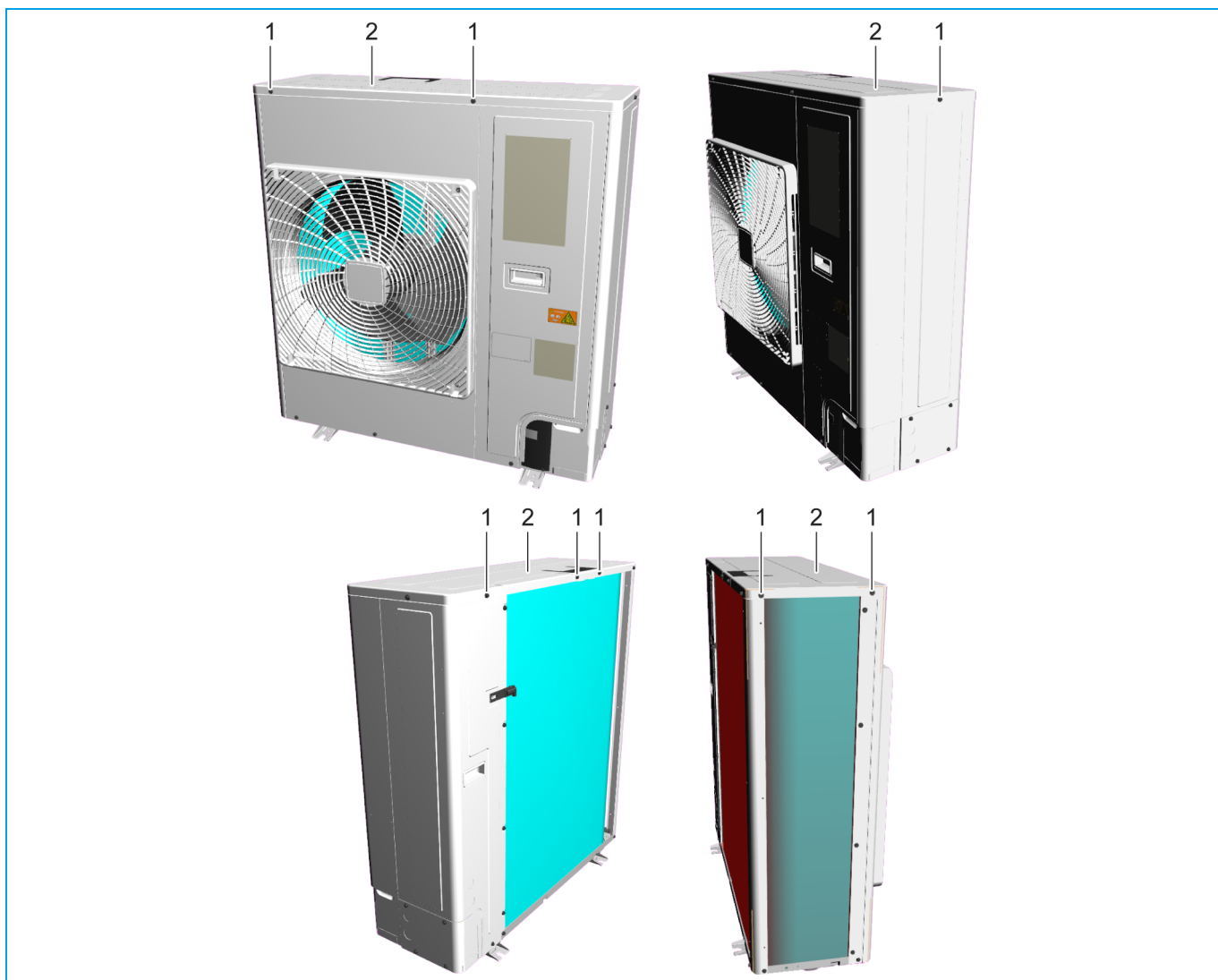
Figure 3-3: Removing the top plate assembly
