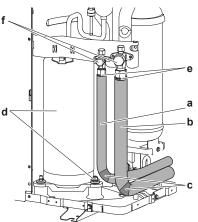
6 If the outdoor unit is installed above the indoor unit, cover the stop valves (f, see above) with sealing material to prevent condensed water on the stop valves from moving to the indoor unit
