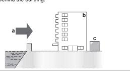
If the outdoor unit is exposed to direct sea winds, install a windbreaker.
