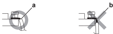
a Strip wire end to this point b Excessive strip length may cause electrical shock or leakage.
