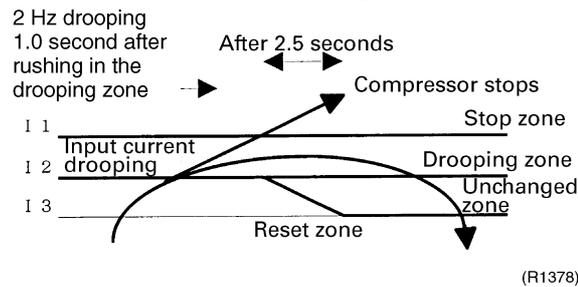
When a “stop current” continues for 2.5 seconds after rushing on the stop zone, the compressor operation stops.
