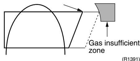
When operating with insufficient gas, although the rise of discharge pipe temperature is great and the electronic expansion valve is open, it is presumed as an insufficient gas if the discharge pipe temperature is higher than the target discharge pipe temperature.
