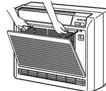
**3. Take off the air purifying filter, Photocatalytic deodorizing filter.**
