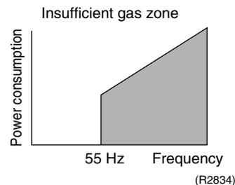
With the conventional function, a power consumption is weak comparing with that in the normal operation when gas is insufficient, and gas insufficiency is detected by checking a power consumption.
