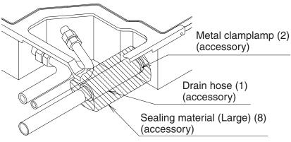
Fig. 27 (Rightward piping)
