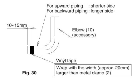
2. Insert the drain hose (1) and the elbow (10) to the root of the drain socket. Tighten the metal clamp (2) within the taped range of hose inserted tip with the torque 1.35±0.15N·m (135±15N·cm). (Refer to Fig. 25, 26, 27, and 31)
