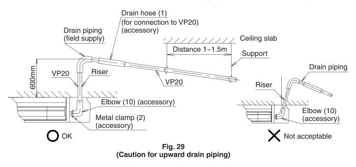
Make sure to use the attached drain hose (1) (for rightward piping), the elbow (10) (for upward and backward piping) and metal clamp (2).
