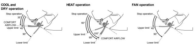
• In swing operation during cooling operation, the upper flap does not move. This is not malfunction. When swing operation is stopped, the upper flap angle changes according to the lower flap angle.
