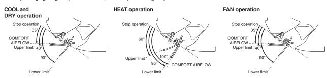
• In swing operation during cooling operation, the upper flap does not move. This is not malfunction. When swing operation is stopped, the upper flap angle changes according to the lower flap angle.
