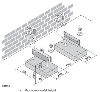
If the unit is installed on brackets to the wall, install the unit as follows:
