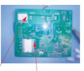
Power transistor Diode bridge (TRM, TPM, IGBT, IPM, SPM, etc.) (Diode bridge, Rectifier stack, etc.)
