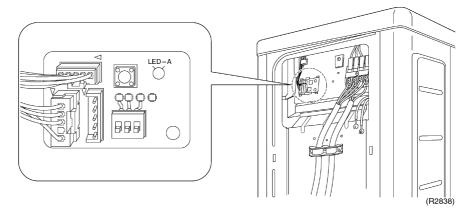
The outdoor unit has one green LED (LED A) on the PCB. The flashing green LED indicates normal condition of microcomputer operation.
