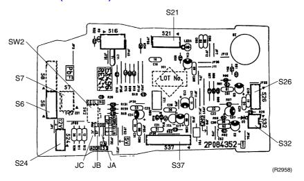
PCB (2): Power Supply PCB (indoor unit)
