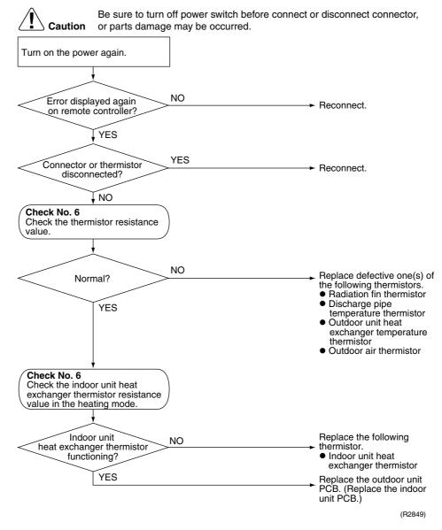
P4: Radiation fin thermistor из: Discharge pipe thermistor
