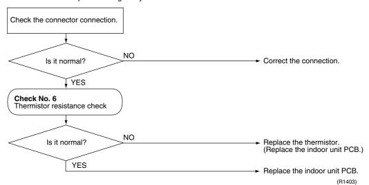
Eq: Indoor heat exchanger thermistor Eg: Room temperature thermistor
