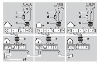
2 user interface control. (2 remote controllers control 1 indoor unit)
