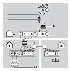
Group control. 1 user interface controls up to 16 indoor units (all indoor units operate according to the user interface).
