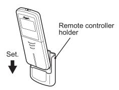
• To remove, pull it upwards.
