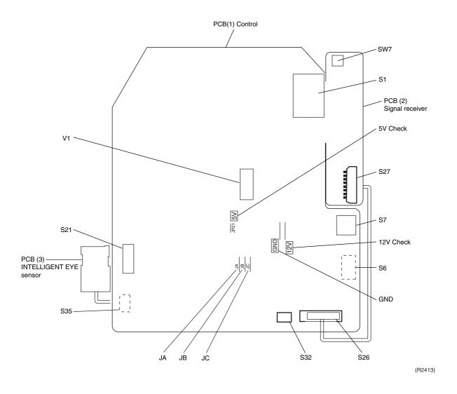
PCB Detail PCB(1): Control PCB
