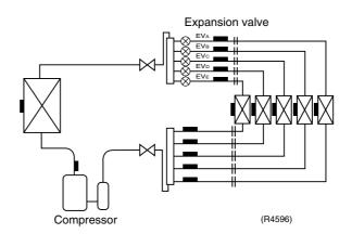
Note: Expansion Valve: In Case of 4 port model.....EVA-D, 5 port model.....EVA-E.
