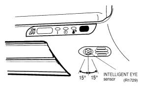
■ Gently push and slide the sensor to adjust the angle. Aim so that the sensor is pointing to the center of the room, or to the part of the room that is most frequently used.
