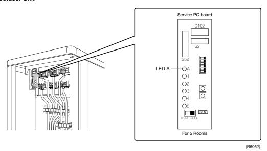
There are green and red LEDs on the PCB. The flashing green LED indicates normal equipment condition, and the OFF condition of the red LED indicates normal equipment condition. (Troubleshooting with the green LED)
