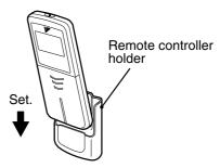
• To remove, pull it upwards.
