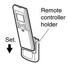
To remove, pull it upwards.
