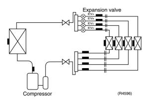
Note: Expansion Valve : In Case of 3 port model.....EVA-C, 4 port model.....EVA-D
