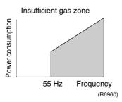
With the conventional function, a power consumption is weak comparing with that in the normal operation when gas is insufficient, and gas insufficiency is detected by checking a power consumption.
