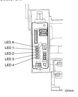
There are green and red LEDs on the PCB. The flashing green LED indicates normal equipment condition, and the OFF condition of the red LED indicates normal equipment condition. (Troubleshooting with the green LED)
