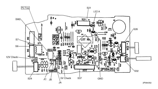
PCB Detail PCB (2): Power Supply PCB
