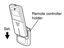
• To remove, pull it upwards.
