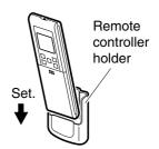
To remove, pull it upwards.
