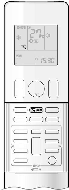
ECONO operation is a function which enables efficient operation by limiting the maximum power consumption value. This function is useful for cases in which attention should be paid to ensure a circuit breaker will not trip when the product runs alongside other appliances.
