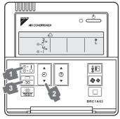
Remote control for VRV BRC1A62
