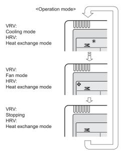
When air conditioner and HRV unit are connected via duct
