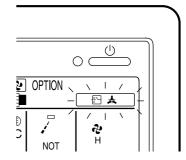
Press the operation mode selector button of the controller that you wish to designate as the master remote controller. Then designation is completed. This remote controller is designated as the master remote controller and the display showing " (changeover under control) vanishes. The displays of other remote controller show " changeover under control).
