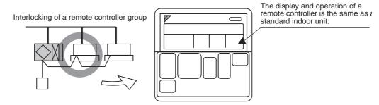
Number of units connectable in case of a remote controller group
