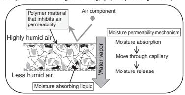
Polymer material that inhibits air permeability that treated on the surface of the heat exchanger element restrains air permeability.
