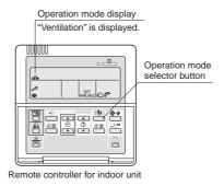
• Each time you press the operation selection button, the operation mode display will change as shown in the figure below.
