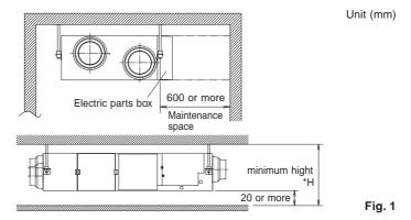
Select the \*H dimension such that a downward slope of at least 1/100 is ensured as indicated in "9 Installation".
