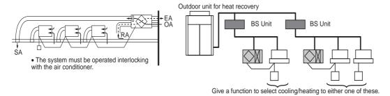
If above setting is not made, the detection of correct temperature is not available and automatic judgment on proper cooling or heating cannot be made when the temperature in the ceiling gets higher than indoor temperature. Poor heating or shortage of the amount of humidification may result.
