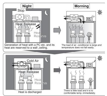
In case of interlocking operation with an air conditione
