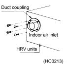
Use the provided screws and install the flange on the HRV units.
