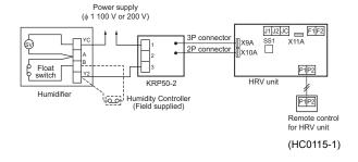
2 KRP50-2 can also be connected to SkyAir indoor unit for the interlocked operation with HRV units.
