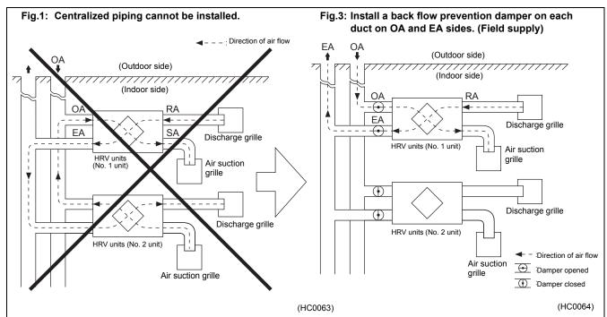
In the above duct system diagram, if a damper is not provided and No.1 unit is operated with No.2 unit being stopped, the air flows in the direction indicated by a broken line, the amount of the air supplied from outside to OA side is decreased, and the air is discharged from the discharge grille of EA side.
