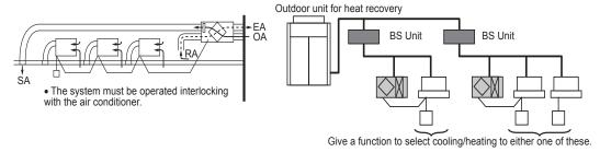
If above setting is not made, the detection of correct temperature is not available and automatic judgment on proper cooling or heating cannot be made when the temperature in the ceiling gets higher than indoor temperature.
