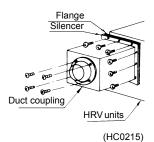
Insert the duct into the duct coupling and wind round the commercially available aluminum tape, etc. to prevent the air leakage.
