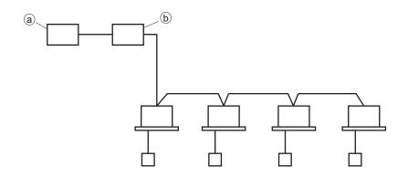
You can perform the normal operation, take off the malfunction contact point and unified operation/stop by contact point, all by connecting this unit with the unification adapter for computerized control. For further details, ask your DAIKIN dealer.
