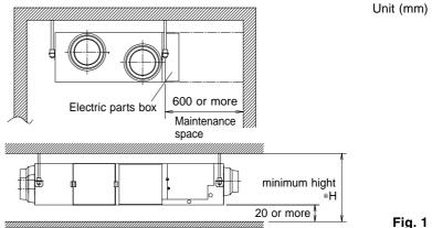
Select the \*H dimension such that a downward slope of at least 1/100 is ensured as indicated in "9.5 Drain Piping and Water Supply Work".
