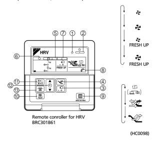
③ Air flow rate changeover button Air flow rate can be changed over to " & " [Low] mode or "♣" [High] mode,
