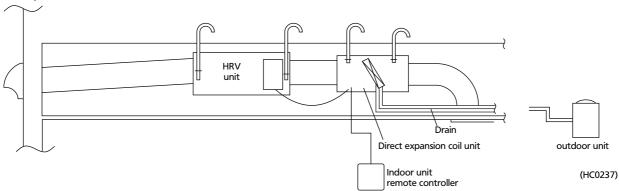
The direct expansion coil helps to recover approx. 100% of exhaust air heat and prevents unpleasant draft. It can also operate as an air conditioner.
