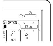
Press the operation mode selector button of the controller that you wish to designate as the master remote controller. Then designation is completed. This remote controller is designated as the master remote controller and the display showing " (changeover under control) vanishes.
