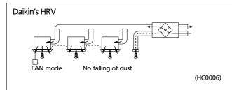
Dust does not fall off from the air filter because the air supply fan of the interlocked indoor unit remains activated even when the HRV is operated independently.
