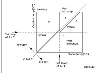
1 zone: Fresh air supply is heated up by indoor air in heat
