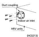
3. Use the provided screws and install the flange on the HRV units.
