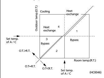
1 zone: Free cooling (cooling by outdoor air) in bypass mode.\*
