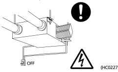
Electric shock may result. Before servicing the unit, always shut off power.
