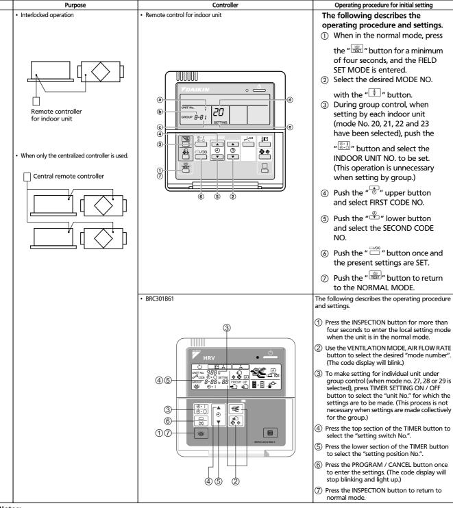
When you make several field settings to one (or one group of) indoor unit(s), the item ② to ⑥ of the above setting procedure should be repeated and it should be terminated to the "normal display" by the procedure of item ⑦ as last.
