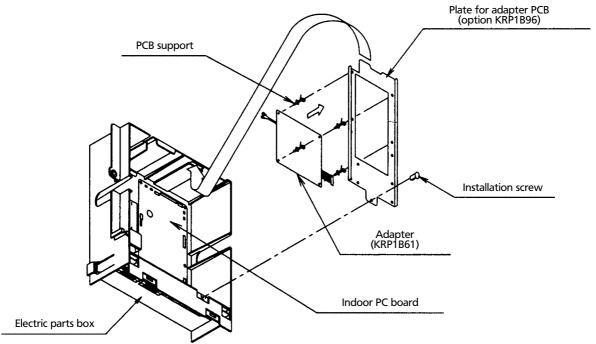
NOTE: A separate plate is needed to install the adapter PCB.
