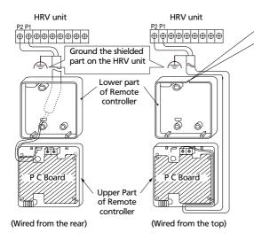
4. Reattach the upper part of remote controller. Be careful not to pinch the wiring when attaching.
