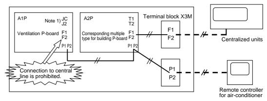
• In case of a central control, operation ON/OFF can be done separately by each zone. (In this case, zone interlocked setting must be kept as the factory setting (17. 08. 01).)
