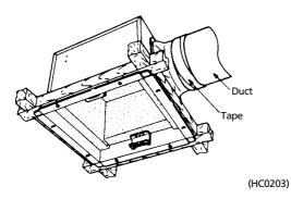
2. Install the ceiling board, providing a clearance of 2 to 5 mm between the flange and the board. (If no clearance is provided, maintenance of the unit cannot be performed.)
