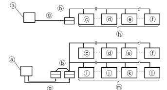
• When using 2 central remote controllers
