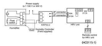
2 KRP50-2 can also be connected to SkyAir indoor unit for the interlocked operation with HRV units. Or to be connected and used for the adapter for outside air preheater.
