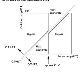
Ventilation mode is individually determined by the original formula of HRV with the temperature sensors.
