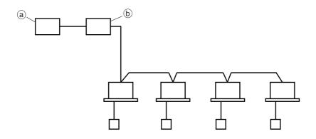
You can perform the normal operation, take off the malfunction contact point and unified operation/stop by contact point, all by connecting this unit with the unification adapter for computerized control. For further details, ask your DAIKIN dealer.
