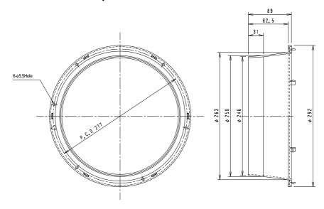
Material: Polystylene (Flammability: UL94V – O)
