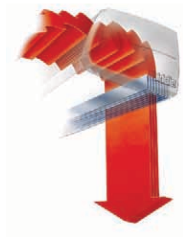
Daikin-Biddle air curtain with patented rectifier grille – separation efficiency up to 90%
