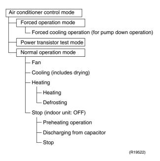
Note: Unless specified otherwise, a dry operation command is regarded as cooling operation.
