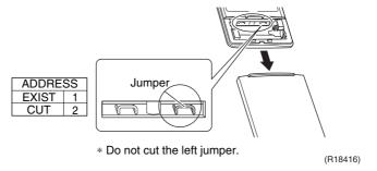
Replace the remote controller if you cut the jumper on the left side.
