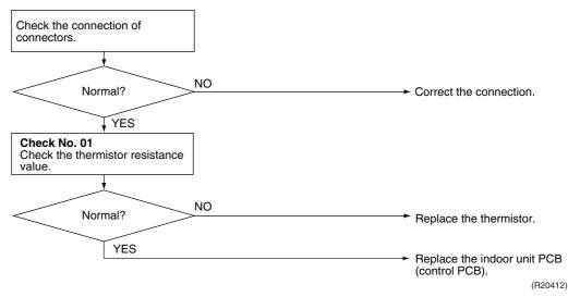
६५ : Indoor heat exchanger thermistor ६९ : Room temperature thermistor
