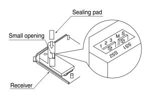
After completing setting, seal off the opening of the address switch and the MAIN/SUB switch with the attached sealing pad.
