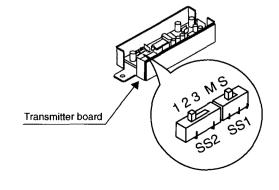
$\ensuremath{\mathfrak{D}}$  Setting the address of wireless remote controller (It is factory set to "1")
