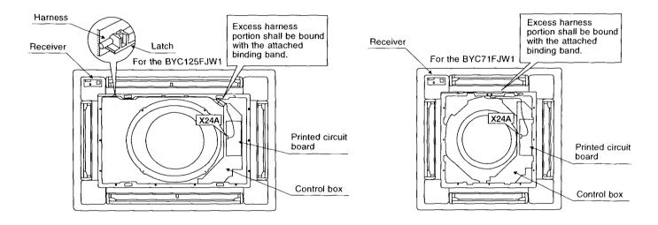
(7) Install the cover of the indoor unit control box and the suction grille to the decoration panel.
