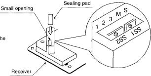
After completing setting, seal off the opening of the address switch and the MAIN/SUB switch with the attached sealing pad.
