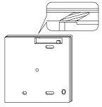
Cut off thin area (hatched area) with nippers or the like, and then remove burr with a file or the like.
