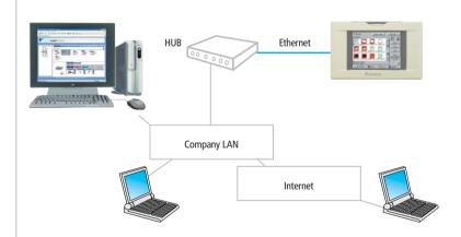
Set up is necessary to receive malfunction notifications via e-mail. Also, the location to be accessed must have an SMTP server. Consult the administrator of your company's LAN for detailed information on the required settings.
