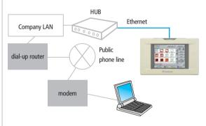
Using a modem and a dial-up router, the intelligent Touch Controller can be accessed from a remote location not connected to the company LAN. Consult the administrator of your company's LAN for information on setting up a dial-up router
