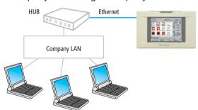
Network setup is necessary to make connections from a company LAN. Consult the administrator of your company's LAN for information on required settings
