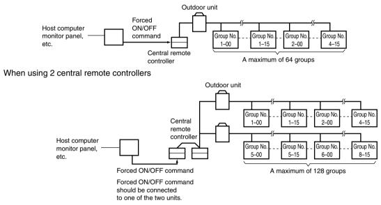
(The central remote controller and the separately sold remote control adapter circuit board or group remote control adapter cannot be used together.)
