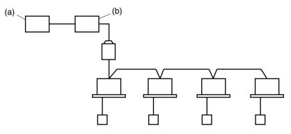
You can perform the normal operation, take off the malfunction contact point and unified start/stop by contact point, all by connecting this unit with the unification adaptor for computerized control. For further details, ask your DAIKIN dealer.
