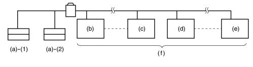
With two central remote controllers, centralized control (indoor units) is possible from different locations.
