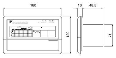
When using this unit an electric parts box of KJB311A is required. For installation, a steel electric parts box to be embedded is mandatory.
