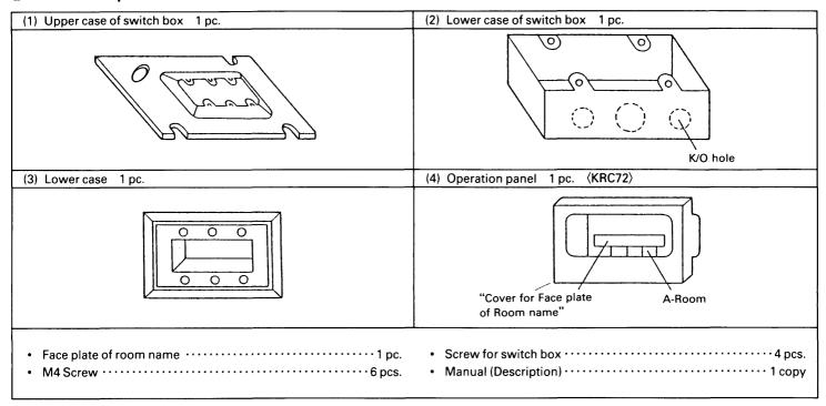
Attention When using this kit, please prepare the P-board (print circuit board) set of remote control (KRC73) of the same number as that of the air conditioners (indoor unit) to be controlled.
