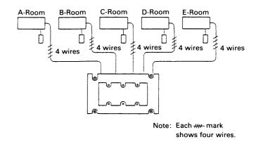
When connecting the wire, please utilize the three of knockouts (K/O) respectively provide for each of upper and lower side of the lower case of the switch box.
