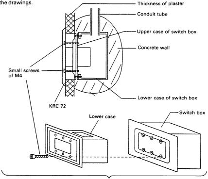
Connecting method of KRC 72 lower case with the switch box. According to the drawing shown in the above, the M4 small screws shall be driven at the respective six holes of the case and box.
