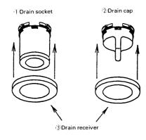
2 Insert drain socket and drain caps into their matching drain hole; Drain socket ① into drain hole B and drain caps ② into drain hole C and D. After insertion, turn them about 40° clockwise.
