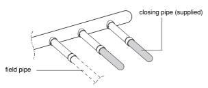
For connecting the field piping to the inlet of the liquid header: Depending on the connection side, attach the expander pipe (supplied) and the closing pipe (supplied).
