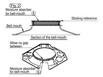
(4) Apply the insulation for bell-mouth (6) on the back of the bell-mouth. See Fig.3
