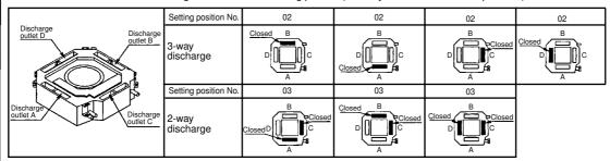
Work on the sealing materials and the fixed tapes for sealing material according to the air outlet number to be closed.
